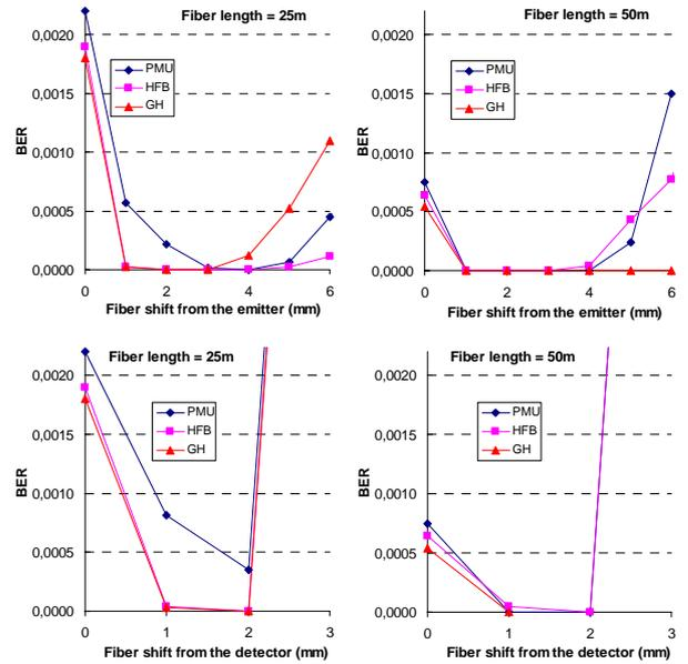
Figure 5: BER versus fiber shift from the emitter and from the detector for lengths of 25m and 50m.
