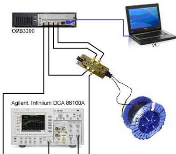
Figure 1: Schematic of the experimental set-up to implement the methods to obtain BER and eye diagrams versus transmission data rate.
