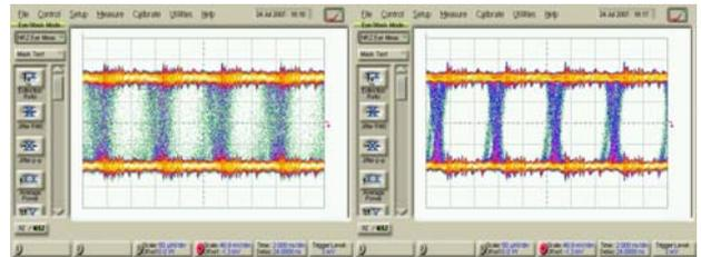
a) Fiber close to emitter      b) Fiber at 1mm from emitter
