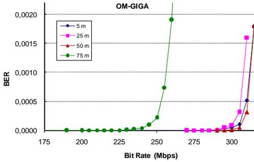
Figure 3: BER versus data rate for OM-GIGA from Optimedia for 5m, 25m and 50m fiber lengths.
