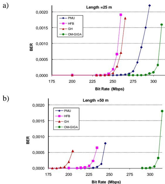
Figure 2: BER versus data rate for PMU, HFB, GH and OM-GIGA. a) Length = 25m. b) Length = 50m.
